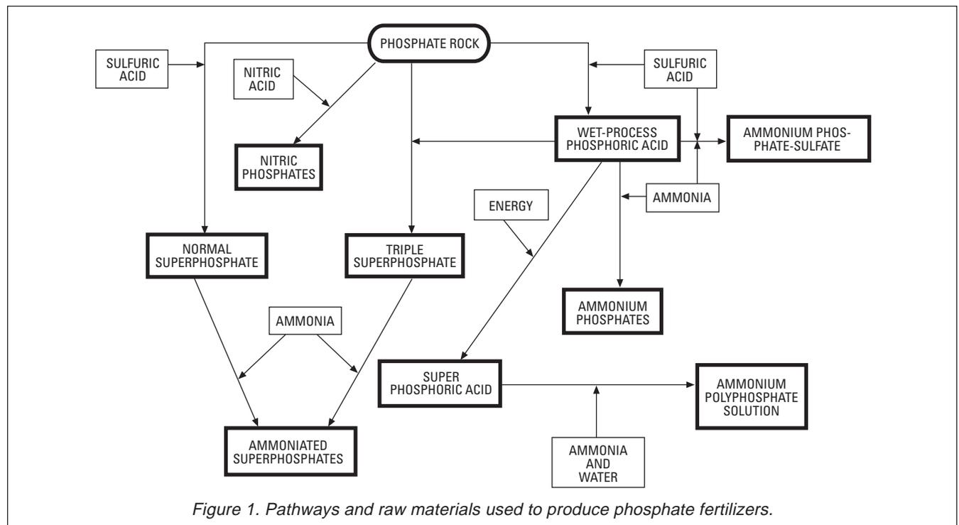
Figure 1. Pathways and raw materials used to produce phosphate fertilizers.
